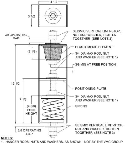
2. STANDARD FINISH: HANGER BOX - PAINTED, POWDER COATED OR GALVANIZED STEEL.
